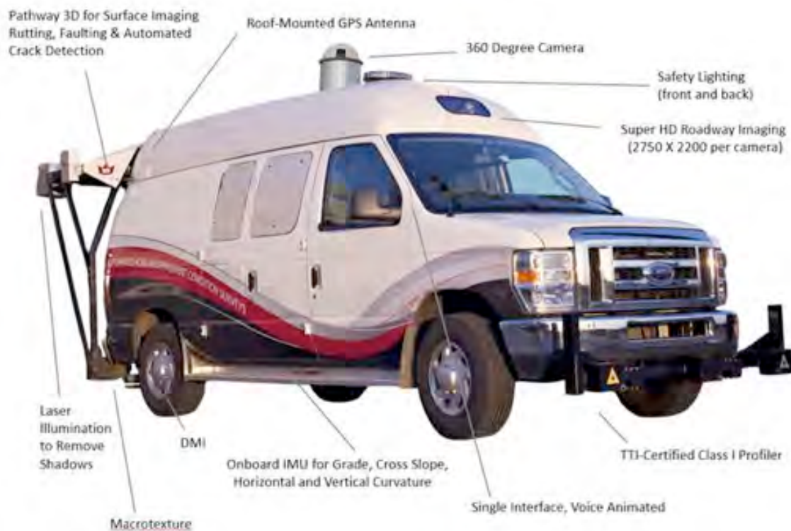
Figure 4-2. Automated Road and Pavement Condition Survey Van
