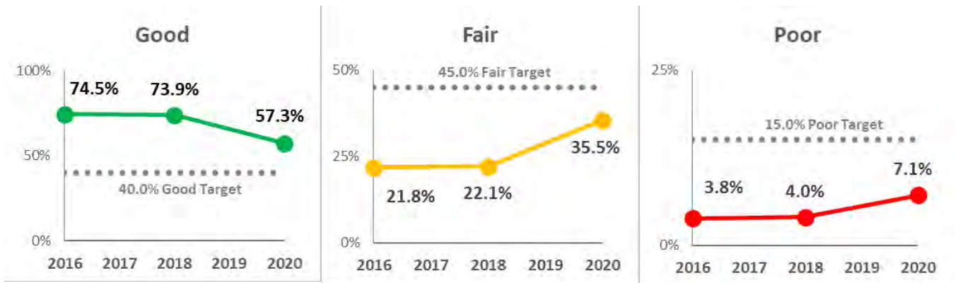
Figure 24 – Condition of Overhead Sign Structures
