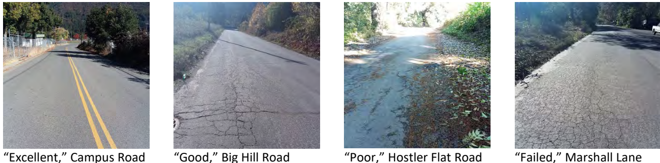
Figure 5. Examples of pavement conditions on tribal roads.
