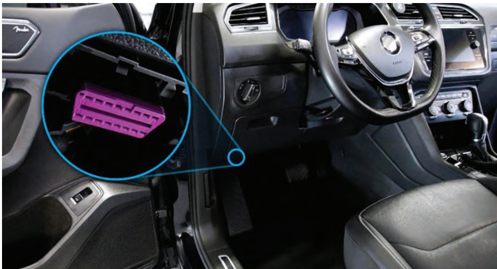
FIGURE 2-5 On-board diagnostics (OBD) refers to the automotive electronic system that provides vehicle self-diagnosis and reporting capabilities for repair technicians and others.
