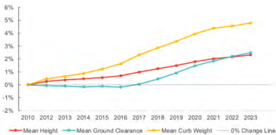
Figure 4. Mean Height, Ground Clearance, and Curb Weight Change in the California Vehicle Fleet from 2010 - 2023
