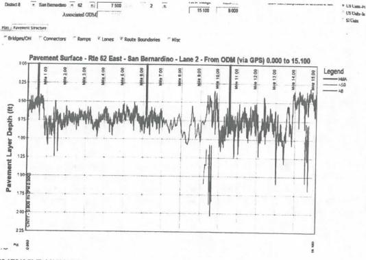
Segment 3 – SBd PM 29.3/33.6- All pavement in the EB #1 lane (graph below) appears to be 0.45' or more with the following exceptions: PM 29.87 shows a depth of about 0.31', PM 33.25 shows a depth of about 0.32' AC and PM 30.0 and 30.45 both show about 0.39' AC.
