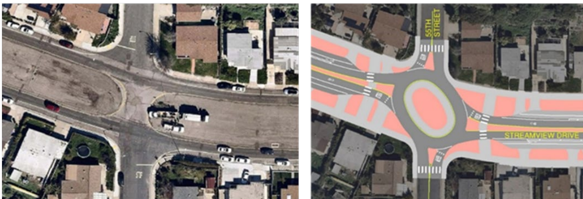
Figure 17: Existing (left) and proposed improvements (right) at the intersection of Streamview Drive and 55 th
