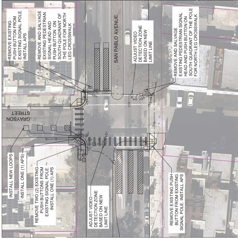
ELECTRICAL IMPROVEMENTS AT GRAYSON STREET AND SAN PABLO AVENUE
