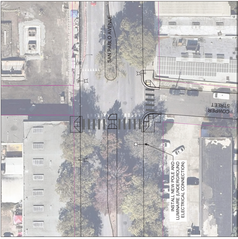
ELECTRICAL IMPROVEMENTS AT COWPER STREET AND SAN PABLO AVENUE
