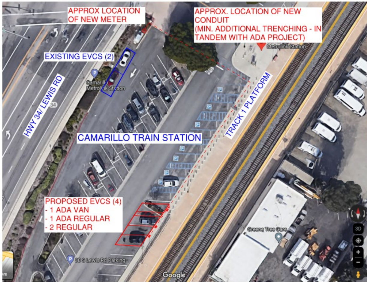
Location 1 EVCS at Camarillo Station
