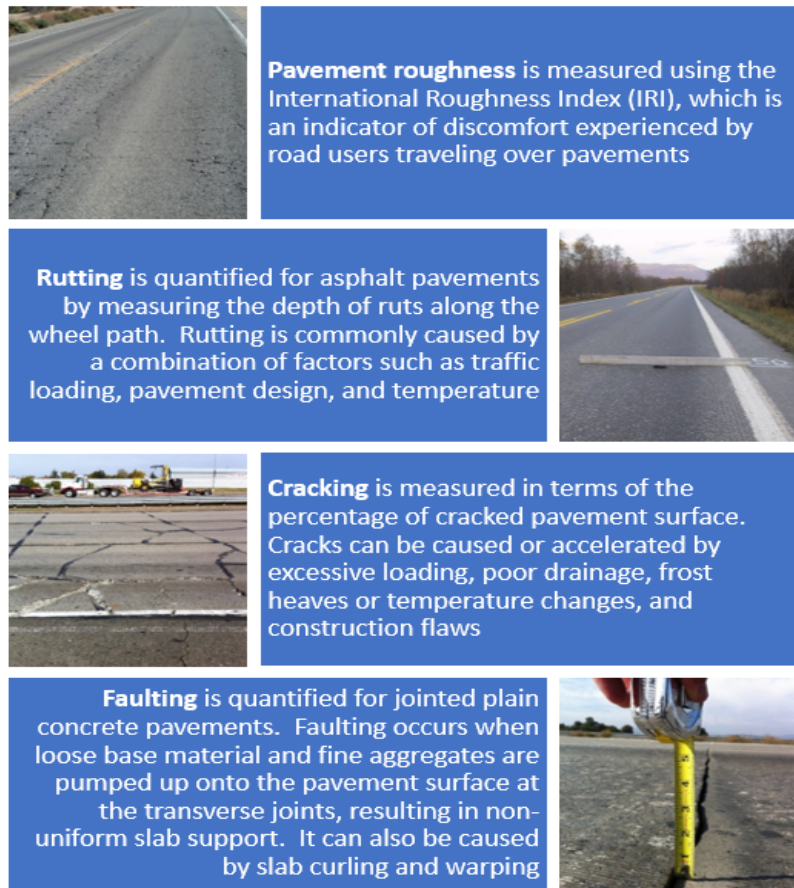
Figure 5-15. Examples of Pavement Conditions
