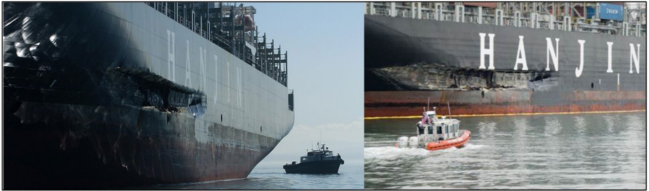
Photos of damage to the Cosco Busan following the allision with a SFOBB Pier W5, 2007
