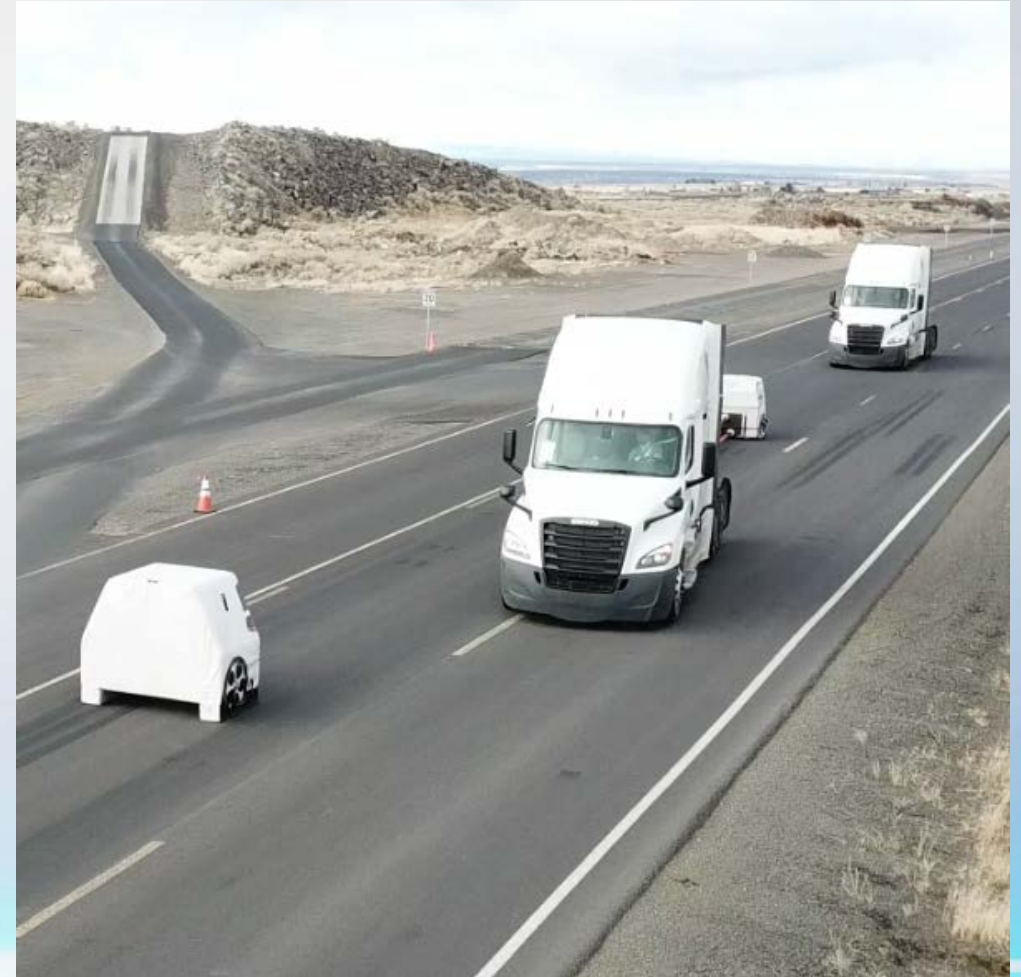
Platooning system safety tests being conducted at Daimler's closed course facility in Madras, OR
