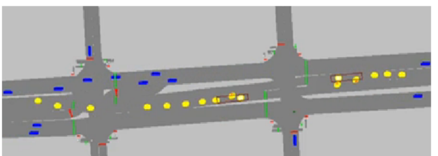
Through TaxiBots (yellow) Passing Loading Bot at ART Station (red rectangles)
